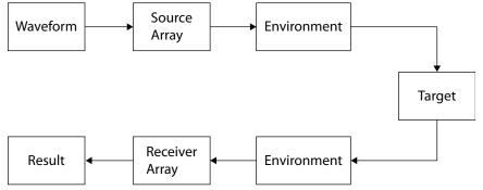
Phased array systems in diverse applications, such as radar, sonar, medical ultrasonography, medical imaging, and cellular phone communication share many common elements including:
