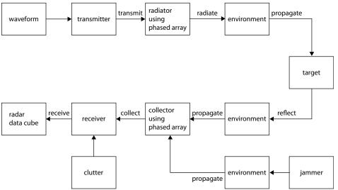
To exploit the advantages of array processing, you must first understand how to model and optimize the performance of each component and operation in a phased array system. This software provides models for all the components of the phased array system illustrated in the preceding figure from signal synthesis to signal analysis.
